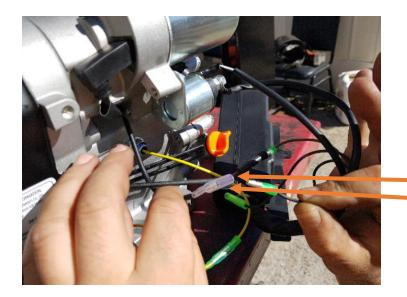
Black (female) from underneath fuel tank, plug into the black (male) from starter box.
