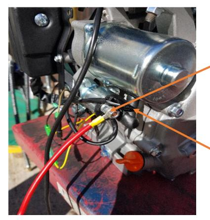
Red Battery Terminal, Place onto silver solenoid coil.
