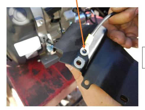
Black battery terminal Place back of starter box when mounting on engine
